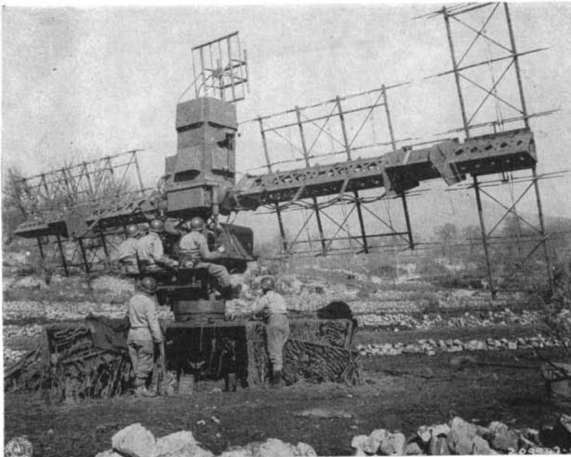
Radar in operation: Radio set SCR-268 with a five man crew is shown in operation on an Italian hillside. The three operators seated on the mount see indications of the airplane echo on cathode ray oscilloscopes. One operator tracks the aircraft in azimuth; another operator tracks in elevation and the third measures the range.
