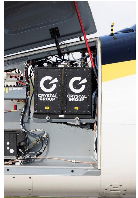
Crystal Group rugged computing systems installed aboard an aircraft to support onboard data processing in a SWaP-constrained environment.
